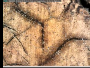
Surface cracks, accumulation of black deposition
