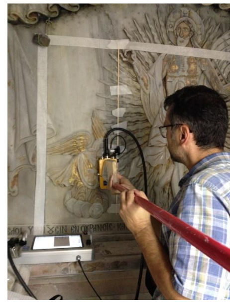
Ground penetrating radar prospection of the opened Tomb
